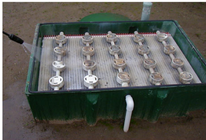
Orenco Advantex fabric filter
