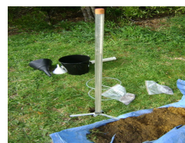
Figure 1: Schematic of a constant head tube permeameter
