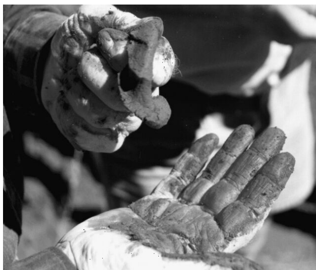
Figure 5 Forming of ribbon from bolus
